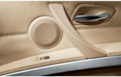
□ **HiFi System Professional LOGIC7** provides truly outstanding sound. 13 loudspeakers and the adjustable surround function create a luxurious soundscape all around you. The central bass concept using subwoofers makes for an authentic bass sound.
