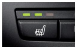
□ Seat heating for driver and front passenger (three settings): Seat surface, sides and backrest are heated and quickly radiate comfortable warmth.
