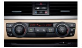
□ Automatic air conditioning, incl. AAR, micro filter, fogging and solar sensors and residual heat button, rapidly provides the desired climatic conditions in the vehicle interior and maintains the selected temperature. With individual temperature control at the front (left/right) and climatised storage compartment in the centre console, incl. rear air vent and air conditioning.
