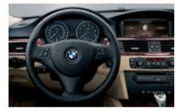
□ Leather sports steering wheel (369 mm diameter), three spokes, incl. gearshift lever handle with chrome trim and handbrake lever handle finished in leather, multifunction buttons for remote control of radio/telephone (both optional); also available without multifunction buttons.
