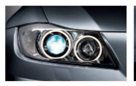
□ Xenon headlights for low and high beam, including four parking light rings and automatic headlight range control, provide much better illumination of the road ahead at night or in poor visibility. □ Adaptive Headlights for improved visibility in
