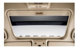
□ **Glass sliding/vent roof,** electric, with wind deflector and comfort opening function via the car's remote control unit, includes reading lights at the front and illuminated vanity mirrors.
