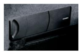
□ **CD changer,** with MP3 decoder, located on the left-hand side of the luggage compartment, holds up to six CDs.
