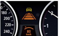
□ Active Cruise Control enables comfortable driving at a pre-selected speed. When driving in columns of traffic, your BMW automatically adapts to the speed of the preceding vehicle and uses its radar sensor to maintain a preset distance. In addition, the braking function ensures that the desired speed is maintained even when driving downhill. (Only available for 325i, 330i and 330d.)
