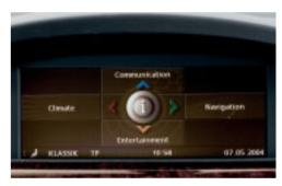
□ Navigation system Business<sup>1</sup>, incl. 2-tuner reception, DVD drive, MP3 decoder and iDrive Controller. Directions are given via arrows displayed on a 6.5" monitor. Additional function: independent ventilation.
